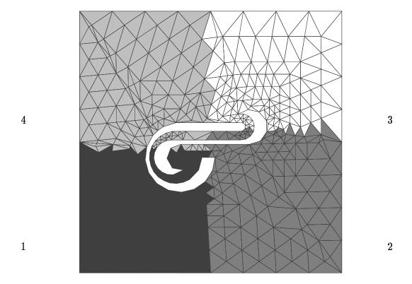
Figure 1 (a) Partitioning of a mesh into 4 subdomains using recursive coordinate bisection
